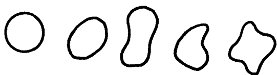
Figure 7 Schematic shapes of the cross-section of gel-derived \text{SiO}_2 glass fibres.
